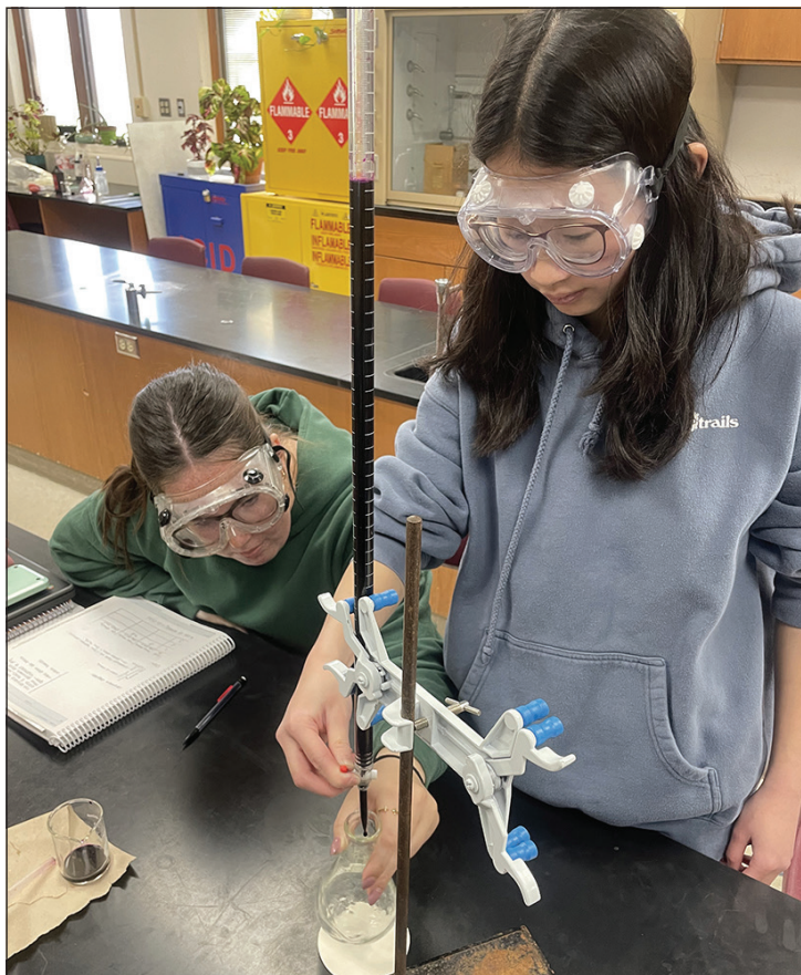
ONTARIO HIGH SCHOOL'S CCP CHEM 130 class practiced analytical lab techniques and applied their understanding of oxidation-reduction reactions. Students completed a redox titration to determine the percent hydrogen peroxide in a solution from a drugstore.
